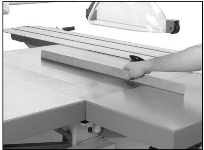
Figure 40. Checking with a straight edge.
